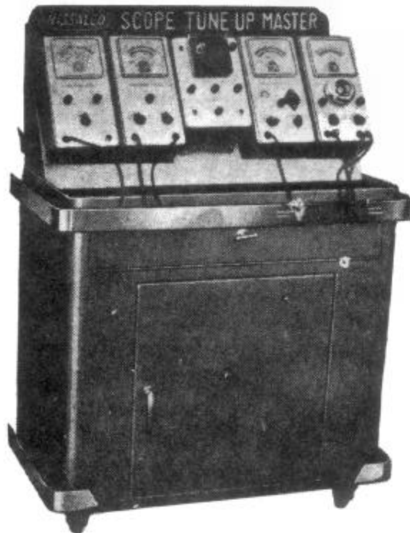
Fig. 2 Motor master tester available for 4, 6, and 8 cylinder engines
