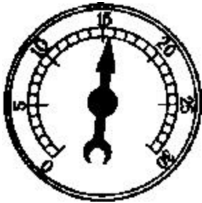
Fig 3. Diagnosing engine by means of a vacuum gauge
