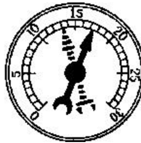
Fig 3. Diagnosing engine by means of a vacuum gauge
